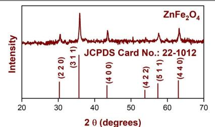
FIG. 1. XRD pattern of ZnFe<sub>2</sub>O<sub>4</sub>.
