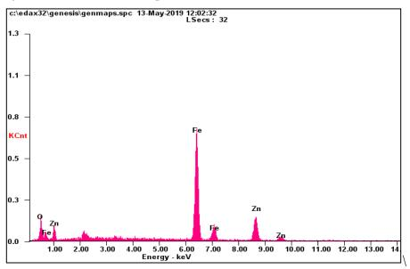
FIG. 3. EDX spectra of ZnFe<sub>2</sub>O<sub>4</sub>.
