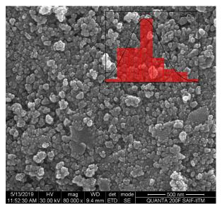
FIG. 4. Particle size distribution of ZnFe<sub>2</sub>O<sub>4</sub>.
